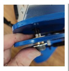
24. Move both pressure arms back in place and put one bolt in only one side loosely (no bushings/washers) – just to hold one pressure arm in place.
