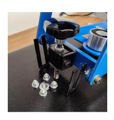
15. Tighten the castle nut and bolt tightly. The long-threaded bolt will go INTO the Black Magnet Bracket
