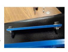
**6.** Fit side link back onto handle and pressure arm.
